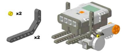
Combine the parts from Steps #1 and #2. Attach the bent beams to the friction pins in the NXT and to the axles from step #1. Use a  $\frac{1}{2}$  bushings to hold the 3-5 bent beam to the axle. Both sides are symmetrical.
