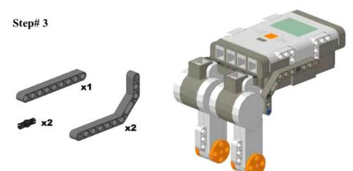
Attach 2 pins to the side of the NXT. Secure Step #2 by attaching a bent beam on both sides of the NXT and a straight beam on top of each motor.
