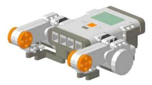
Combine the assemblies from Steps #1 and #2. Attach the bent beams to the bottom of the NXT and the motors to the double pin connectors.
