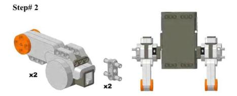
Fasten the motors to the double pin connectors on the bent beams. Then fit a 4 pin connector into the outside mounting beam on the NXT.
