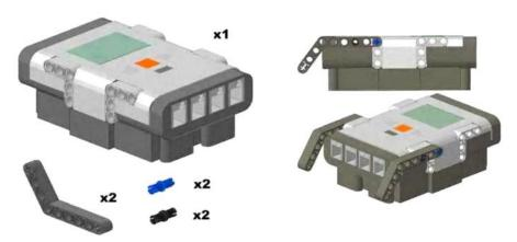
Attach the 2 bent beams to the NXT using a friction pin and an axle pin on each. The shorter portion of the beam should be sticking out from the NXT.
