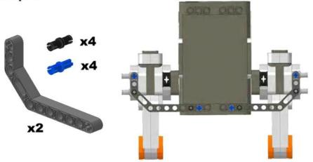
Attach the double bent beam to the 4 pin connector and the NXT using the axle pins and friction pins.
