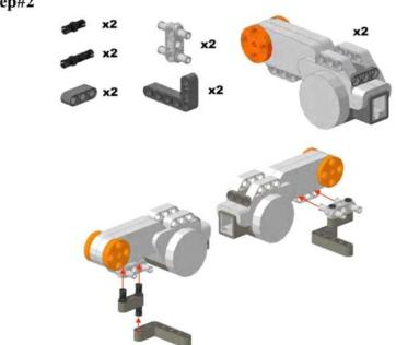
Attach a four pin axle joiner to each of the NXT motors. In 1 hole of the 4 pin connector attach a pin and in the other hole attach an extended pin. Attach the short beam to both pins and the bent beam to the extended pin.
