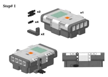
Attach 2 bent beams to the NXT using friction pins. The shorter portion of the beam should be sticking out from the NXT. Insert a double pin connector into this portion.
