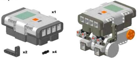
Attach each motor assembly to the bottom of the NXT by the black axle joiner, using a friction pin. Then secure each motor using the bent beam.
