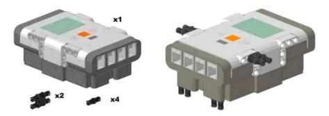
Attach a double pin connector to each side of the NXT. Place 4 pins to the bottom of the NXT in the outside most holes.
