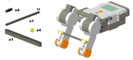
Slide the 12 stud axle through the mounting beams of the motor and secure it in place with  $\frac{1}{2}$  bushings. Use the friction pins to attach the 13 hole beam across the tops of the motors.
