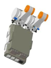
Attach the 4 pins from the perpendicular axle joiners to the bottom of an NXT.
