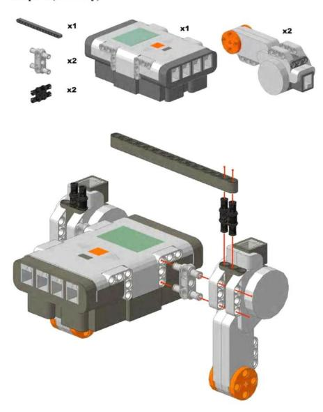
Using 1 beam and 4 connector pegs, attach each motor to the NXt. The left and right sides are symmetrical.
