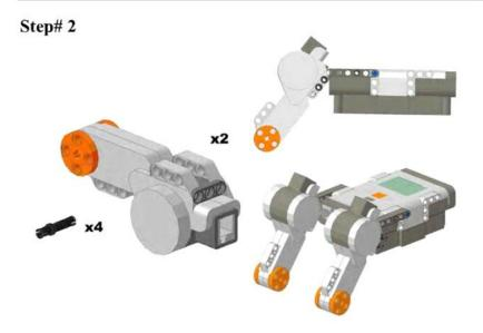
Fasten the motors to the bent beams using the extended pins. Make sure the bent beams are placed in between the 2 mounting beams on the NXT.
